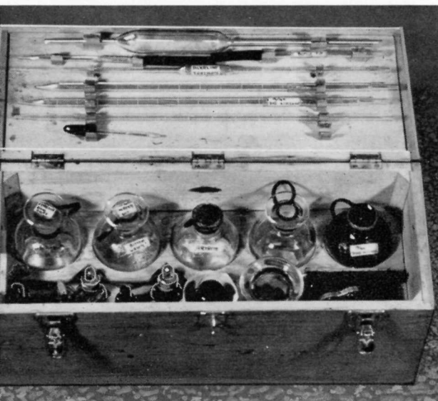
Field kit used for chemical analysis of water.
