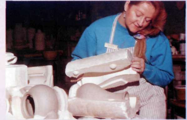
Slip Casting: A plaster mould is filled with liquid clay. The plaster absorbs a thin wall of clay onto it's surface and the surplus slip is poured off.
