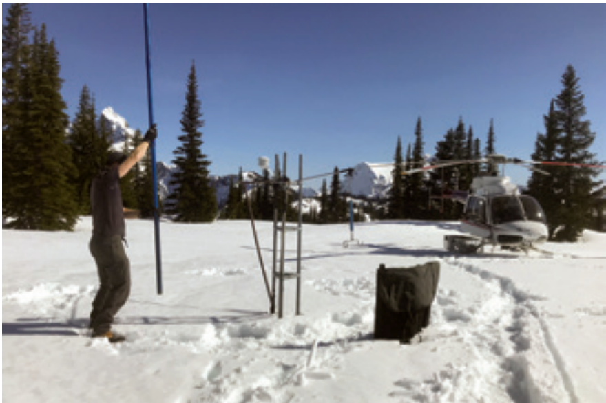
Below: Figure 1 – Malcolm Nicol, snow survey technician with the British Columbia Ministry of Environment performs a manual snow water equivalent verification at Chilliwack River Alpine Snow Water Station. Photo: Ted Litke, BC Ministry of Environment
