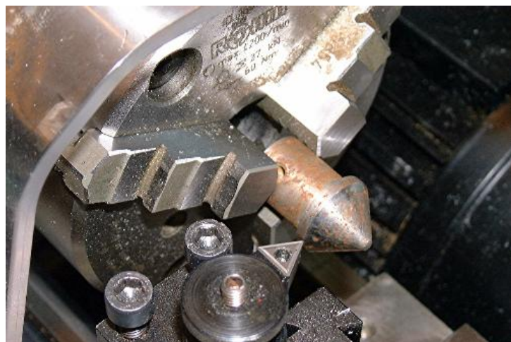
Figure 19: Making the tips on my lathe (Marek-misc: Lathe)
