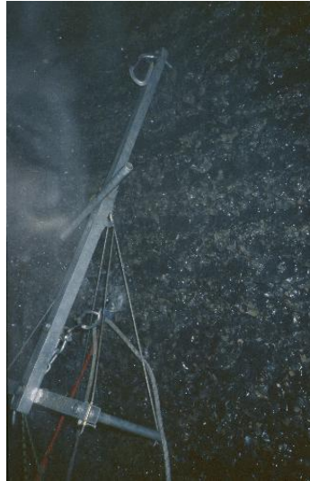
Figure 130: The bolting platform; red "rope" is my connection to the Fifi hook (Marek: CC05-04-0027)
