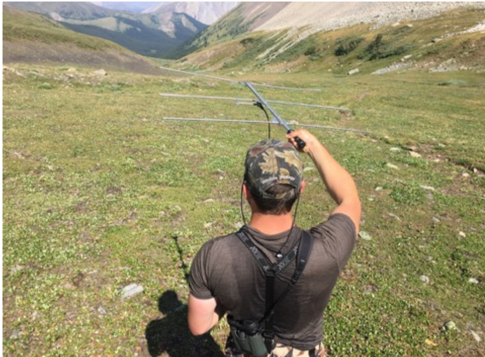
Fig. 5. Locating migratory elk using radio telemetry.
