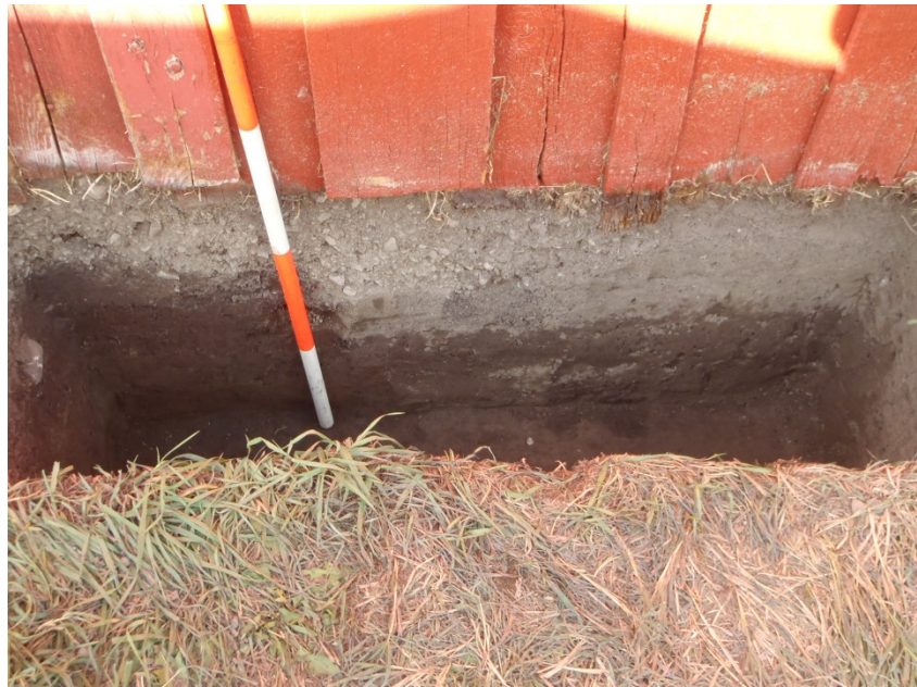
Plate 8 South view of 60 to 70 cm deep tests (Sub-Op's N, L, and M, left to right) shows gravel fill foundation beneath join of two buildings
