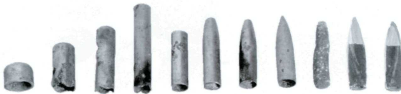
Artifacts showing the different manufacturing stages of a .303 cartridge case (bottom) and bullet (top).
