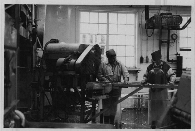
Figure **5C**Salting machine with gravity feed can system for filler (Photo'byauthor)
