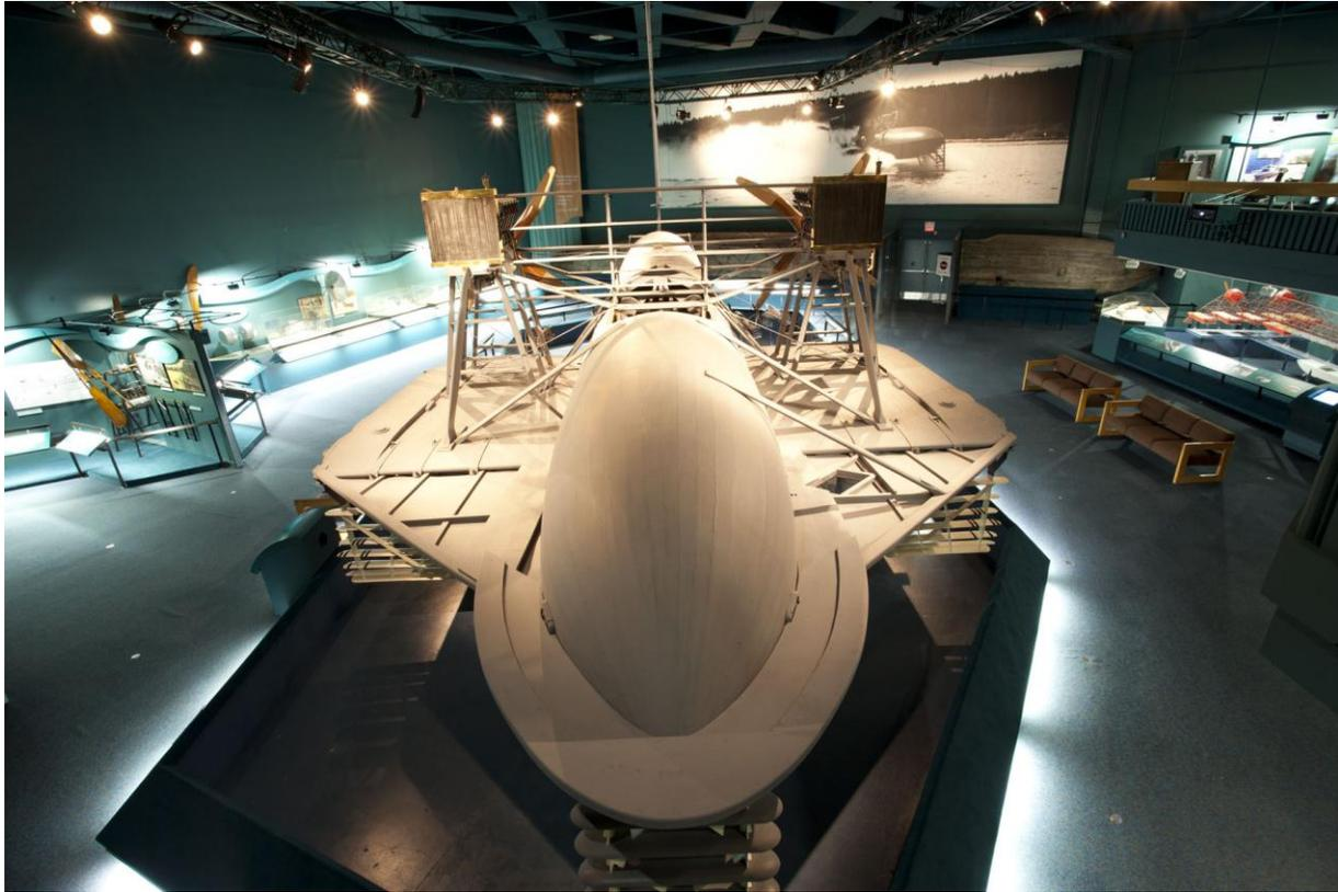
Figure 9: Full-scale reproduction of Bell and Baldwin's marine record-setting hydrofoil boat HD-4 adjacent to the conserved original hull.
