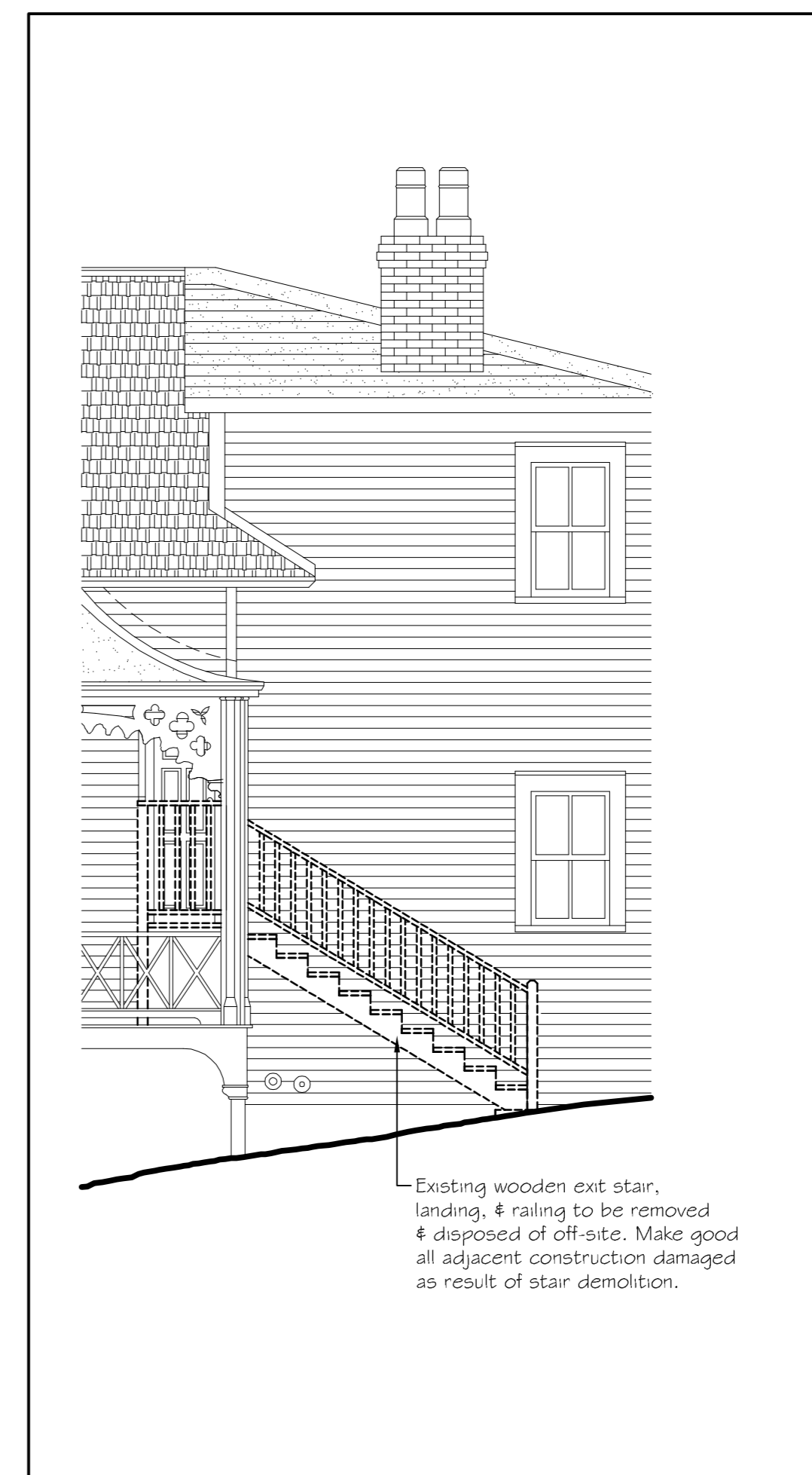
3 Exit Stair Demolition A-402 1:50
