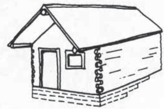
Use of a mud sill to overcome slope
