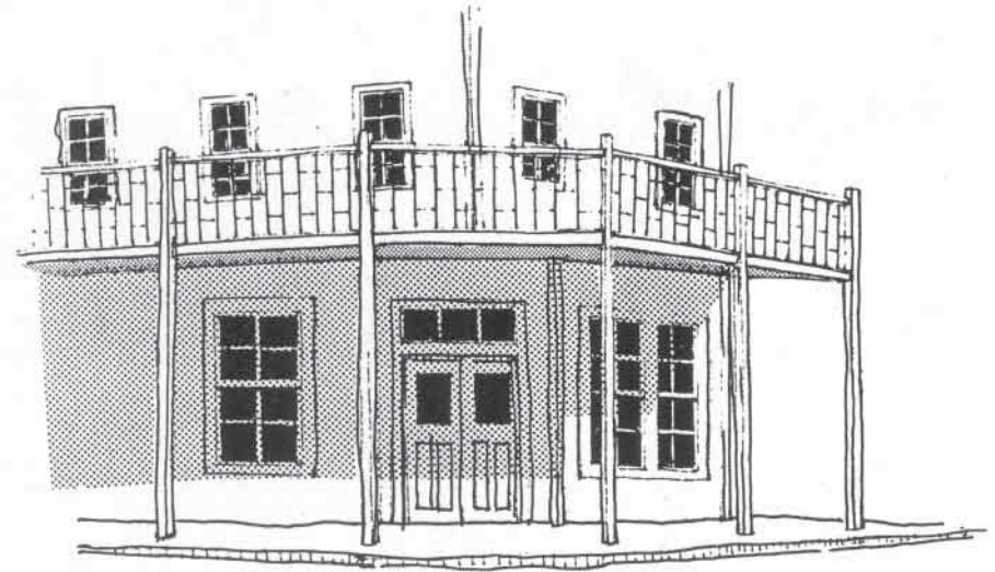
Balcony supported by columns
