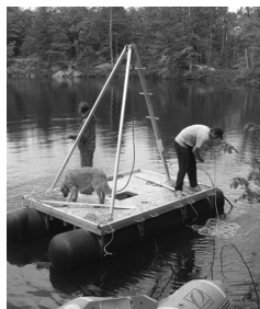
Photo: Douglas Hallett The coring raft at Little Black Lake.
