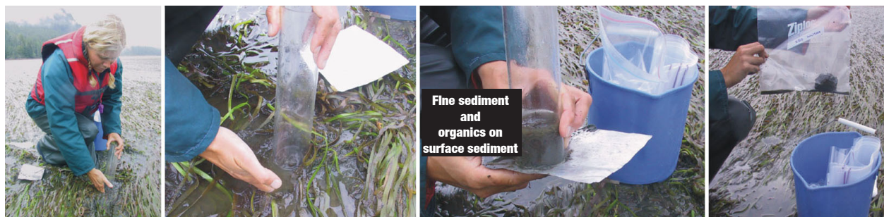
FIGURE 3.5 Sediment field sampling protocol
