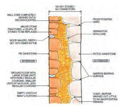
Section of exterior masonry wall showing typical deterioration observed.
