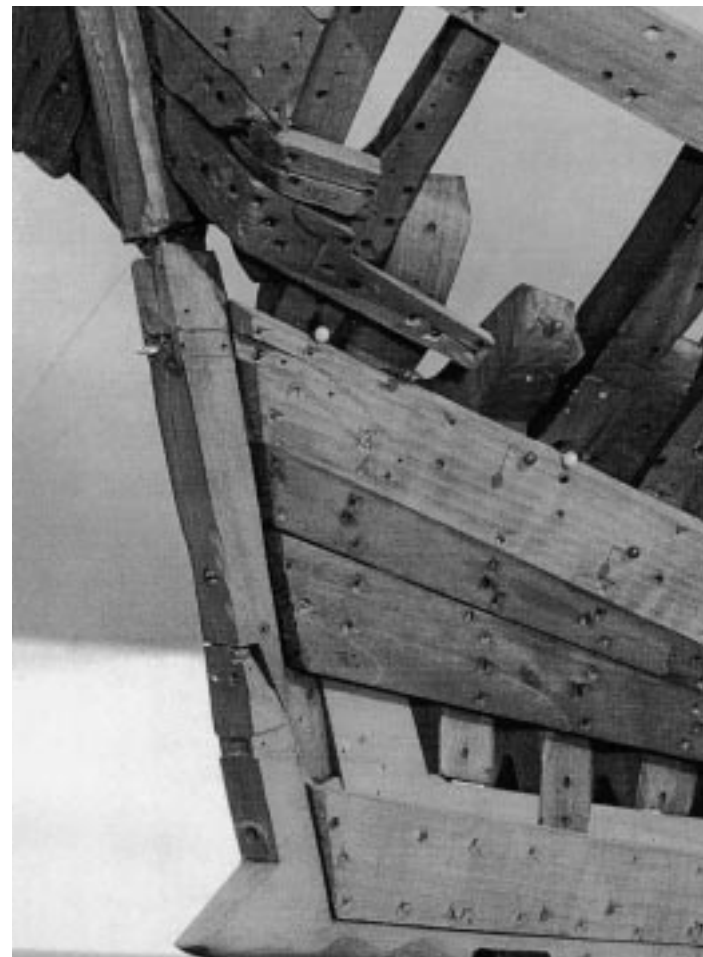
FIG. 18 – Lower starboard stern of the model at the keel and stern post junction, showing carved planks wrapped around the lower end of the fashion piece, creating a seamless link between the transom and starboard side. This was a clever way to overcome weakness and leakage at this critical junction in the square tuck hull (Photo: R. Chan, Parks Canada; RD-1137W).
