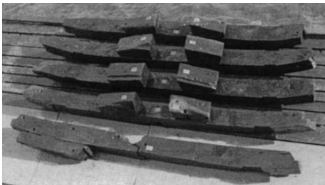
FIG. 12 – After they were raised to the surface for recording, four of the midship floor timbers (1st forward to 3rd aft of the master frame, top to bottom) and eight reinforcing chocks for the main mast step were placed in their original arrangement for this photograph. The second frame from the top is the master frame, with two dovetail mortices at either end. In the foreground, the floor shows the carved-out sump hole cut vertically through it (Photo: R. Chan, Parks Canada; 24M-2056M).
