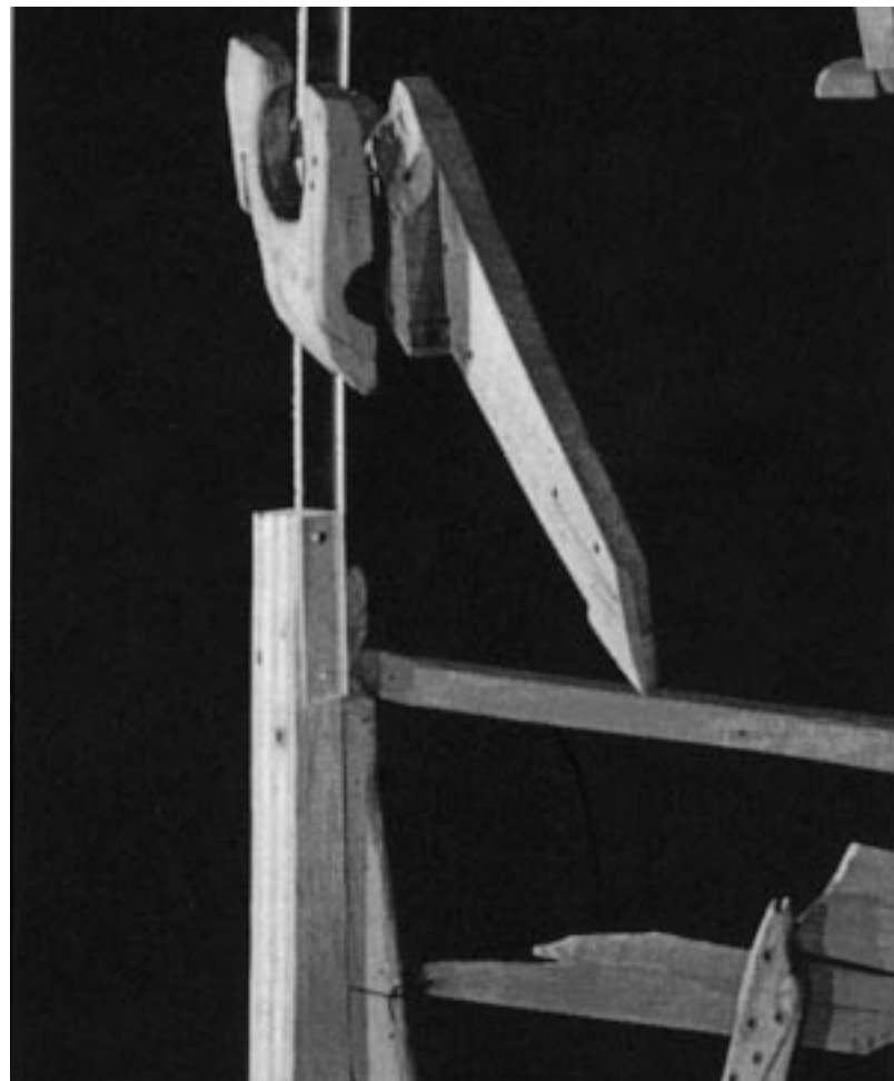
FIG. 27 – Model looking forward, just aft of the stem, showing the two main components of the port side hawse hole assembly ( escobenque ). The outer portion with the large carved hole shows a rounded recess where it overlapped a wale. The inner portion of the assembly, oriented at an angle, was secured over hull framing, thereby reinforcing the bow assembly (Photo: R. Chan, Parks Canada, RD-340X).
