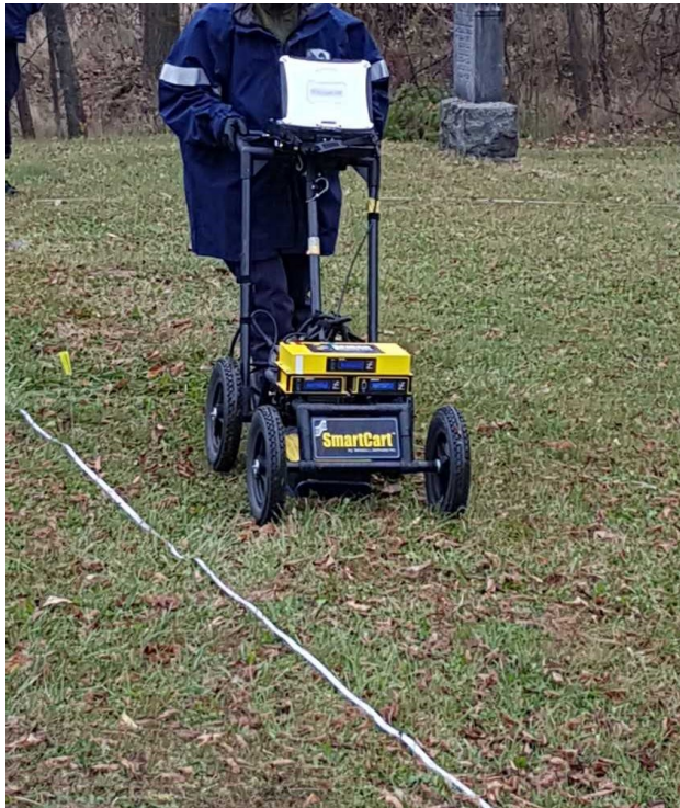
FIGURE 5: A GROUND-PENETRATING RADAR (GPR) UNIT IN-USE AT NEWBORO CEMETERY (PHOTO PROVIDED BY DON ORR).
