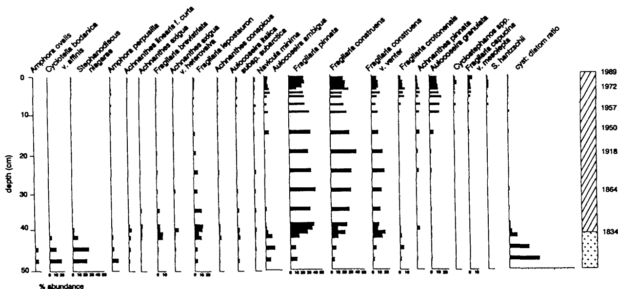
Figure 2.—Summary relative frequency diagram of the most common diatom species recorded in the Upper Rideau Lake sediments. ^{210}\text{Pb} dates are shown to the right. The construction of the Rideau Canal was also delineated in the sediment record by a shift from light brown sediments (stippled) to a dark brown organic gyttja (diagonal lines) as shown to the right of the diagram. The cyst:diatom ratio is a relative measure, expressed as a percentage, following Smol (1985).
