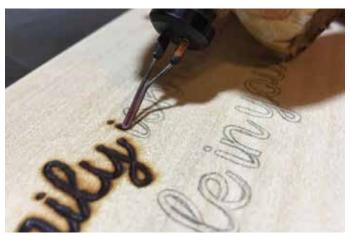
Pyrography or laser etching on wood
