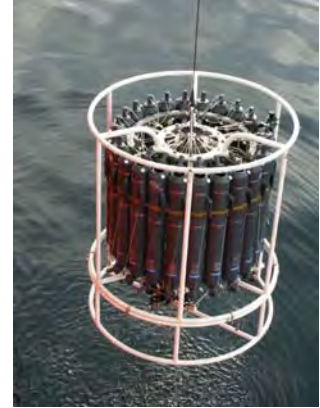
CTD rosette deployed from CCGS Amundsen
