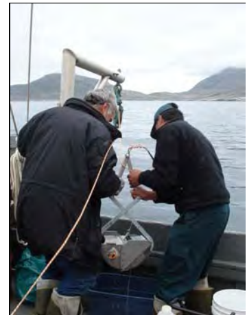
Joe Webb and Jacko Merkuratsuk retrieve the sediment grab sampler
