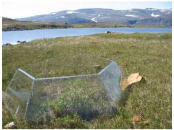
Open Top Chamber to simulate climate warming on wet site – mosses were studied in these mini-greenhouses
