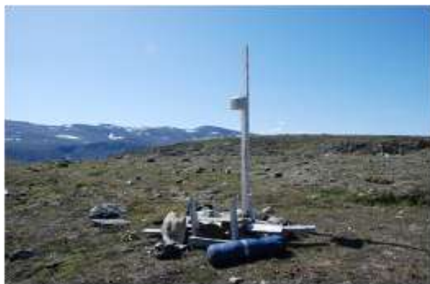
Backup temperature and relative humidity data logger located across from the Nakvak climate station.
