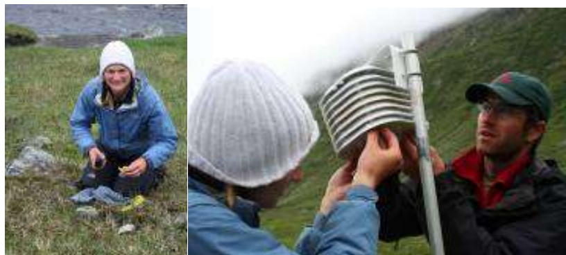
Offloading and resetting data loggers that monitor daily soil temperature (left), air temperature and relative humidity (right) throughout the year.
