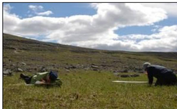
*Researchers using the point frame protocol to sample vegetation in Nakvak Brook*
