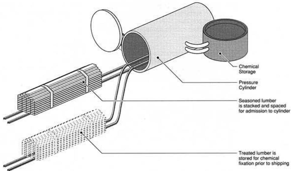
Figure A2.1 Manufacture of pressure-treated wood (CWC, 1995).
