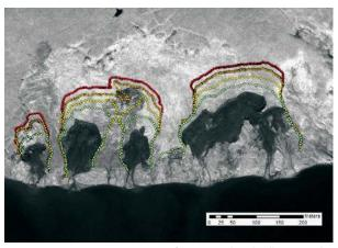
**FIGURE 1.** GPS survey positions of retreating headwalls mapped onto a satellite image. PHOTO: W. POLLARD
