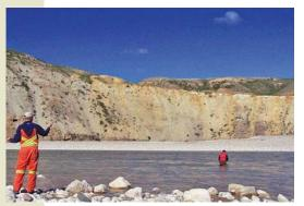
Water survey technicians taking flow measurements on the Hornaday River. PHOTO: WATER SURVEY OF CANADA
