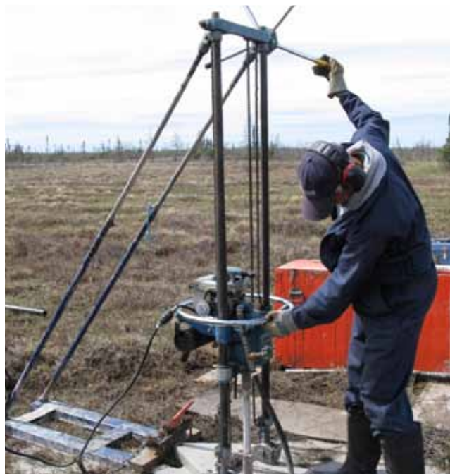
Figure 13: Lightweight drill used for installing thermistor cables.
