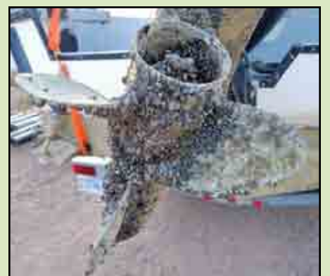
Quagga mussel encrusted motor NPS Photo
