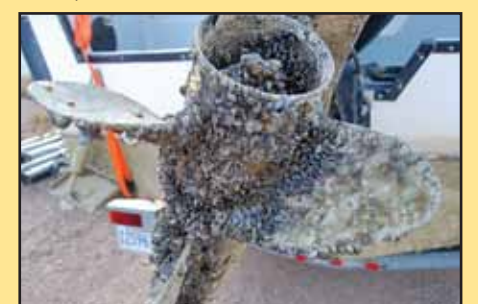
Quagga mussel encrusted motor NPS Photo
