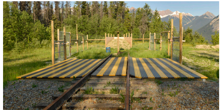
Electric mat experiment at railway crossing mock-up. (© Parks Canada / D. Rafla)
