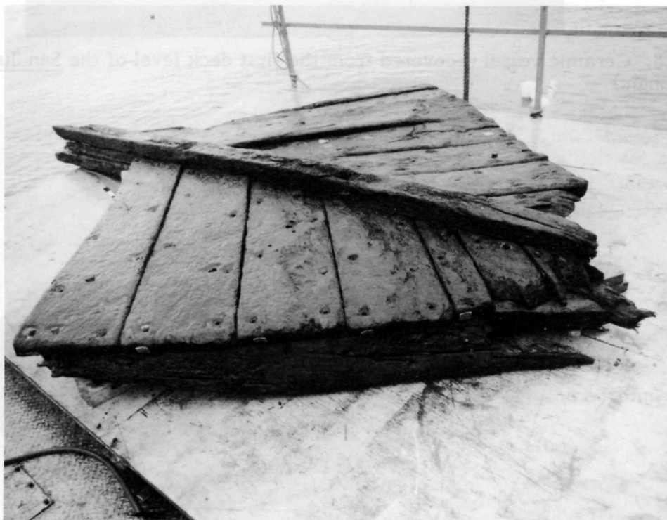
Figure 7. Reassembled transom on the deck of the research barge. (Photo by R. Grenier.)
