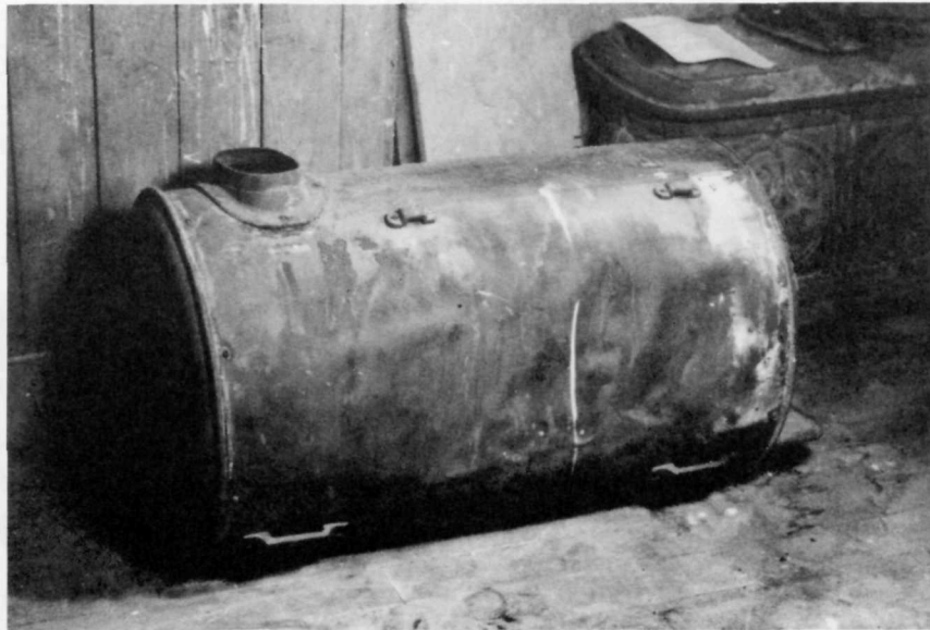
Figure 19. Enterprise camp heater consisting of a metal drum with cast ends, legs and attachment brackets, four brackets for a shelf on top, hearth plate and chimney sleeve. ( One-Room School Collection, Historical Resources Administration, Fredericton, N.B., temporary legislation no. V354-5. )
