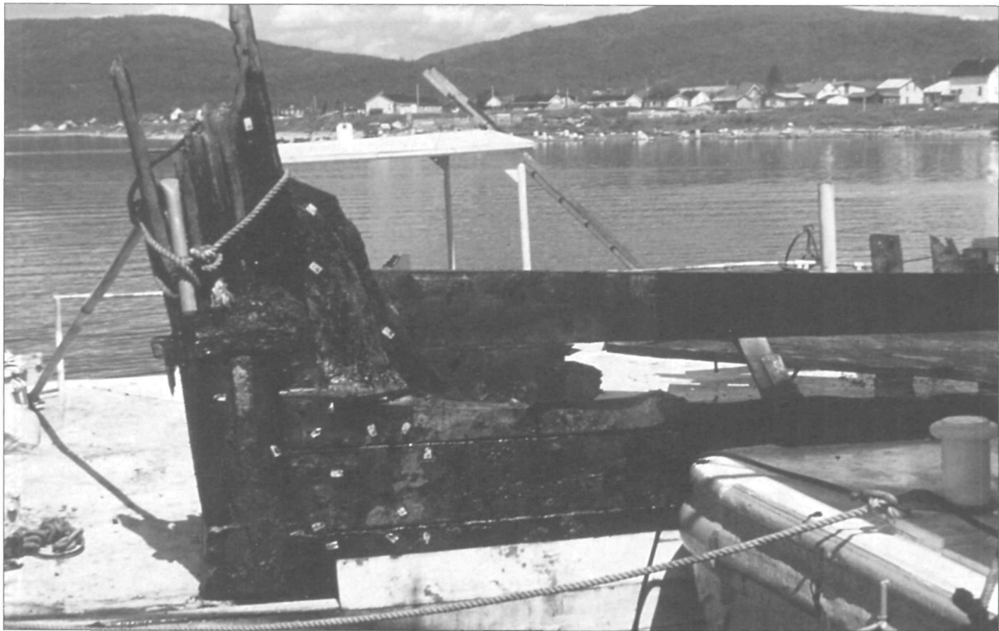
14 Heel of the keel and base of the sternpost of the Machault . Department of Canadian Heritage.
