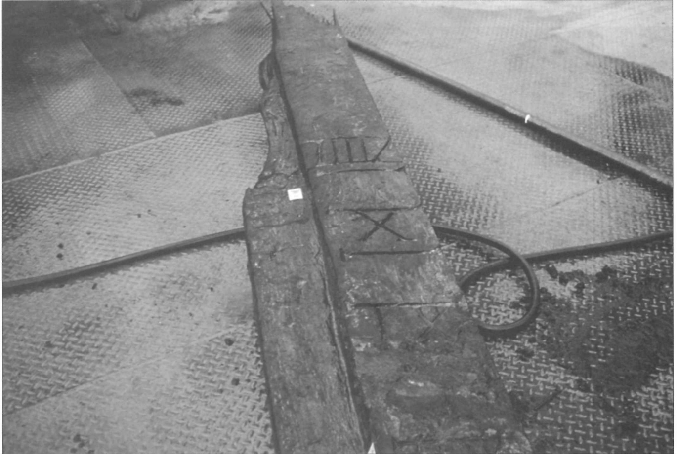
15 Sternpost-rudder of the Machault , with stern draught marks. Department of Canadian Heritage.
