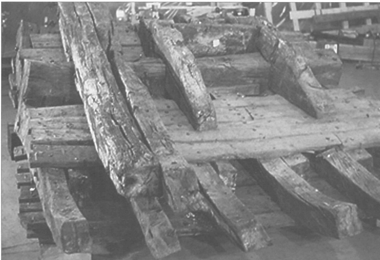
19 Step of the mainmast of the Machault , with interior planking, floor frames and keelson, as recovered from the Restigouche River. Department of Canadian Heritage.
