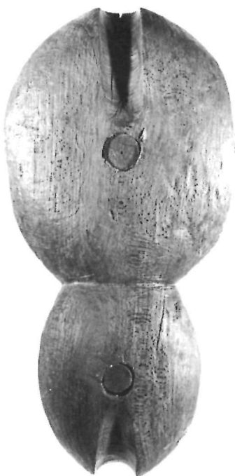
Long tackle block, sometimes called a fiddle block, set up as a pulley
