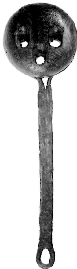
Iron futtock plate attached to a three-hole deadeye
