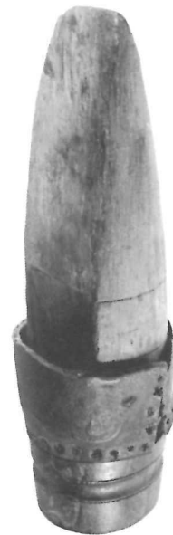
Wooden piston with its leather gasket
