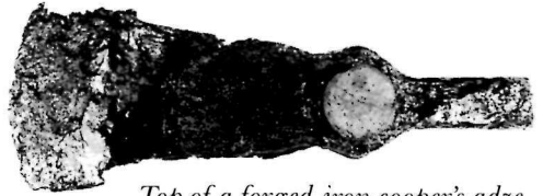
Top of a forged-iron cooper's adze with a secondary working face
