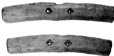
These hardwood caulking-mallet heads were reinforced by metal bands at their ends and by metal bolts on both sides of each handle
